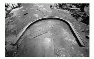
Team Sial Ghogri crafted Arch Support. This conventional technique is a trusted traditional method for providing reliable roof support in underground mining operations. This will also be utilized by WCL to prepare for the International Rescue Competition to be held in Colombia.
